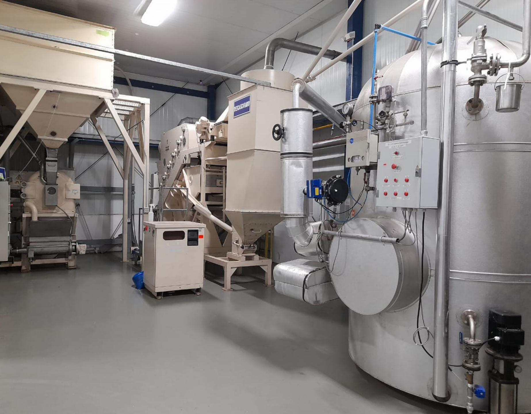
Steam accumulator, Bauermeister 5 exit winnower, silo and Pethhold Heidenauer cocoa nib mill
